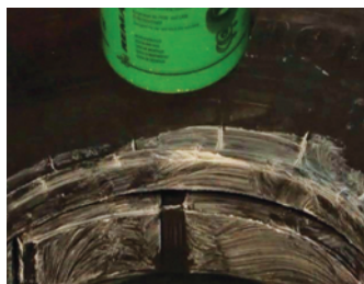
26. Make sure you have tyre soap on the tyre bead also.
