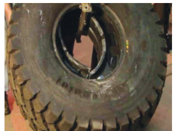
12. If you lift the tyre, gravity will do the work and runflat will drop inside the tyre.
