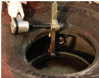
4. If needed, use a bead spreader to improve access into the tyre. A bottle jack could also be used.
