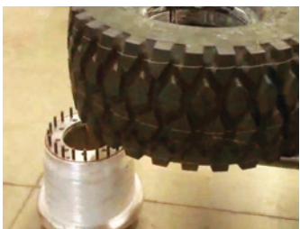
28. Ensure the wheel also has plenty of tyre soap - NB The wheel also has wooden chocks to lift it off the floor.
