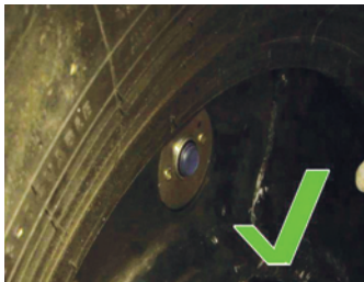
19. Make sure bolt has passed through the locking ring - Be careful not to over tighten.
