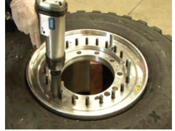
39. Tighten each clamping bolt in short bursts.
