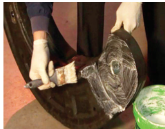
5. Apply tyre soap to the connection faces and the sides of the runflat.
