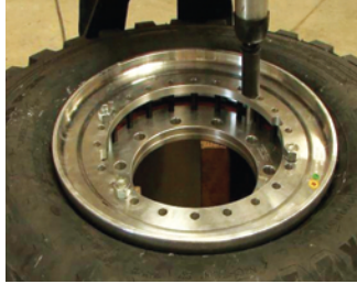
38. Working opposite clamping bolts, one at a time, tighten them so the flange comes together equally.
