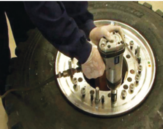
40. Fit the locking nuts and tighten down at least 4 nuts opposite each other using a 24mm socket.
