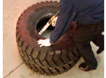
3. Evenly spread the tubes of lubricant inside the tyre.
