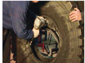
18. Tighten the connection using a 30mm socket.
