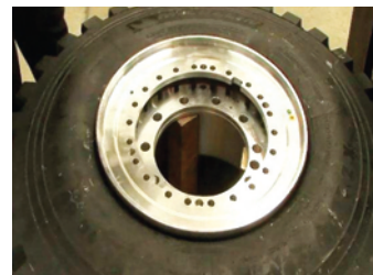
33. Flange aligned on the wheel.
