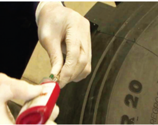
44. Apply some thread sealer to the valve.
