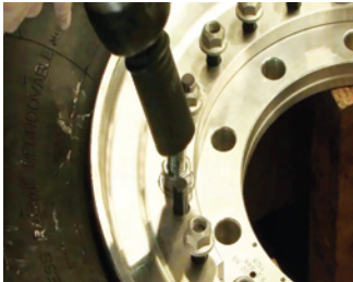
41. You can now remove the clamping bolts and fit the rest of the 22 locking nuts.
