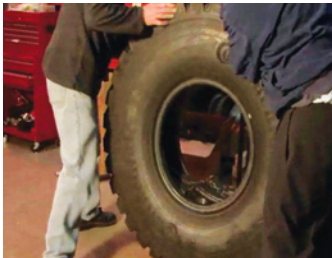
16. Lifting the tyre and rolling it will use gravity to bring together the last connection.
