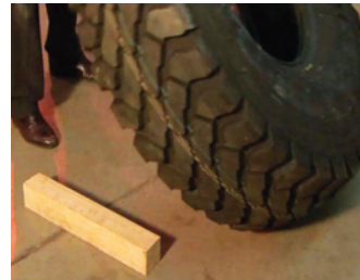
23. Drop the wheel flat. Put in wooden chocks to allow the forks of the lift truck to get access underneath.
