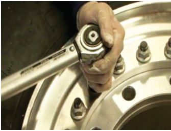
43. Torque the 22 nuts to 217 Nm using this criss-cross method.
