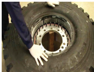
29. Slide the tyre and runflat onto the wheel - NB extra weight may be needed.
